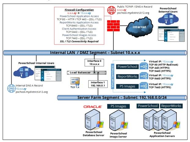
Each corresponding **Virtual Service** will then distribute traffic to the actual PowerSchool server(s) on the 192.168.0.0/24 network. If configuring SSL/TLS termination on the load balancer, the PowerSchool server(s) will accept incoming traffic from the load balancer on native non-secured ports.
