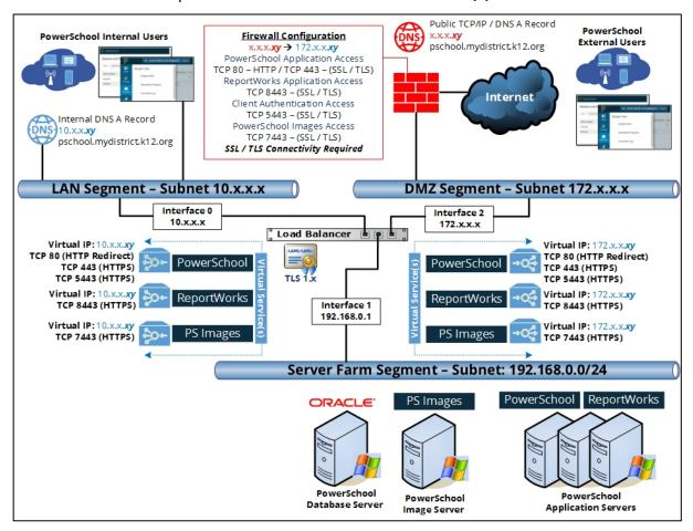
Each corresponding **Virtual Service** will then distribute traffic to the actual PowerSchool server(s) on the 192.168.0.0/24 network. If configuring SSL/TLS termination on the load balancer, the PowerSchool server(s) will accept incoming traffic from the load balancer on native non-secured ports.
